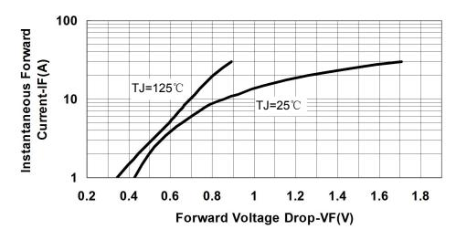
Fig.3-Typical Forward Voltage Drop Characteristics
